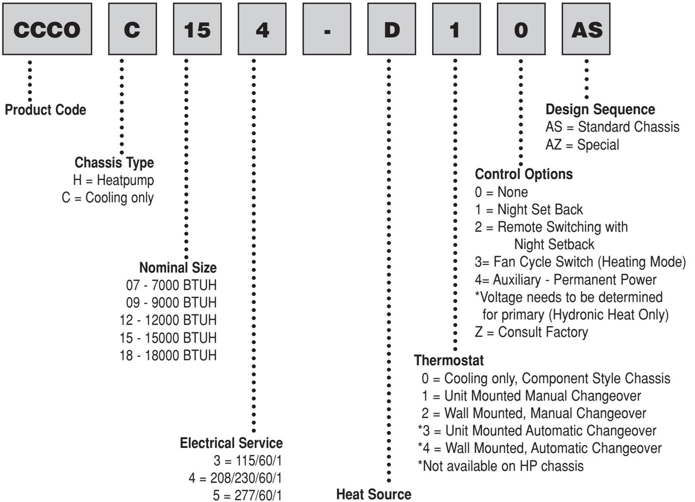
The sample unit coding above indicates a **CNI** Cooling Chassis for replacement of a Nesbitt® Challenger; 15000 BTUH, 208-230/60/1, Hydronic Heat, Unit Mounted, Manual Changeover, No Control Options, Standard.
